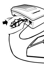
Connect one end of the cord provided with the unit into the PHONE jack of the Super Phone Ringer and the other end into your telephone.
